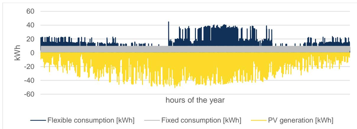
Figure 2: Flexible, non-flexible demand and PV generation for the Spanish pilot site.
