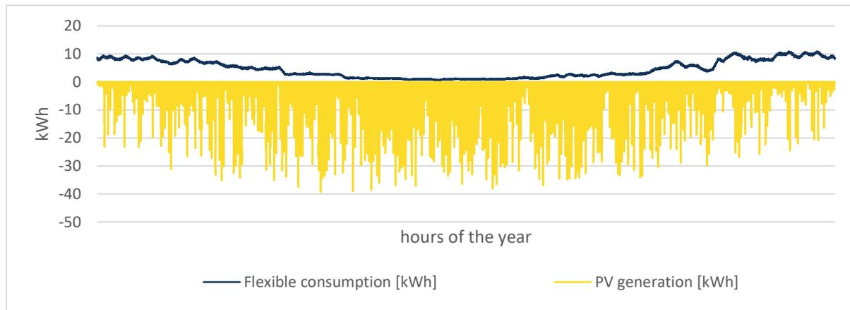
Figure 3: Flexible, non-flexible demand and PV generation for the Belgian pilot site.
