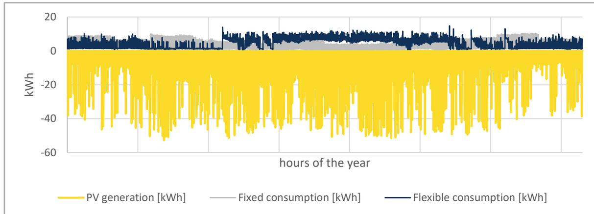
Figure 1: Flexible, non-flexible demand and PV generation for the Austrian pilot site.
